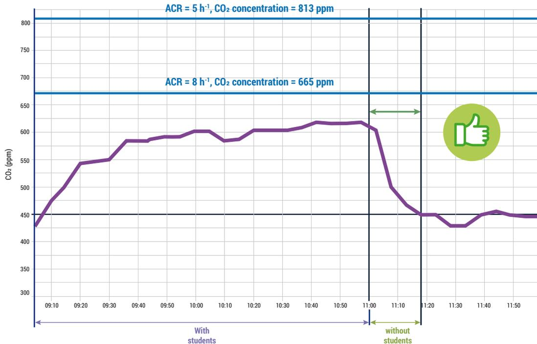
In this example, the classroom has a volume of 142 m<sup>3</sup> and contains 21 students of 10 years of age and one teacher. With this occupancy, more than 5 air changes per hour are recommended. In the adjoining graph, the indoor steady-state CO<sub>2</sub> concentrations corresponding to 5 and 8 air changes per hour are indicated (the latter value is equivalent to conditions for 14 liters per person per second).
