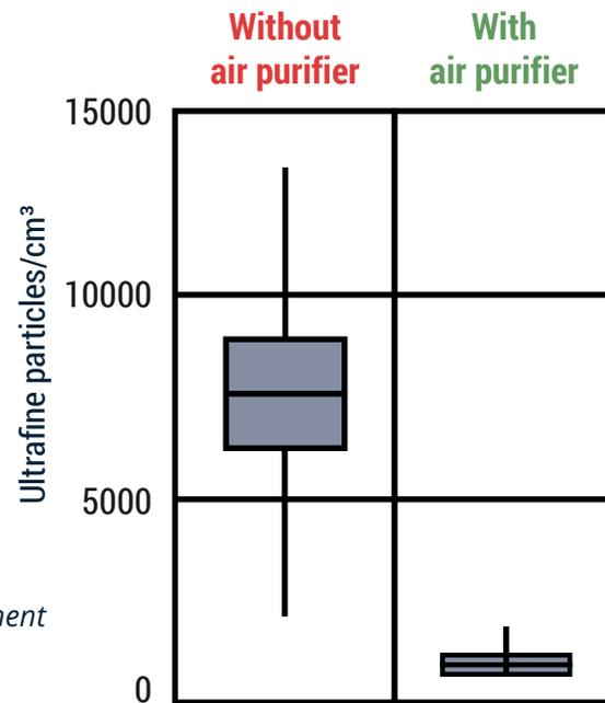
In this example, six air cleaners are installed, each with flow rates of 660 m<sup>3</sup> per hour, in a school gymnasium of volume 430 m<sup>3</sup> (150 m<sup>2</sup> \* 2.9 m).
