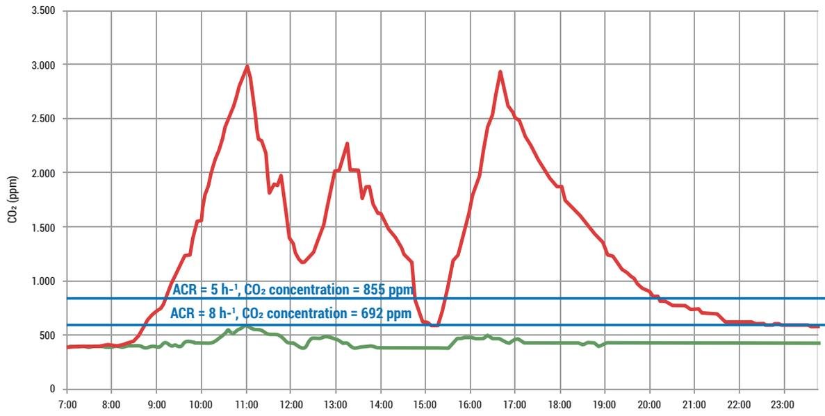
In this example, the classroom has a volume of 148 m<sup>3</sup> and contains 22 students of 14 years of age and one teacher. With this occupancy, more than 5 air changes per hour are recommended. In the adjoining graph, the indoor steady-state CO<sub>2</sub> concentrations corresponding to 5 and 8 air changes per hour are indicated (the latter value is equivalent to conditions for 14 liters per person per second).
